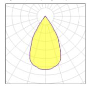
LED CCT 3000 K Lamp type Nominal lamp power 7 W CRI 80 Total flux LOR 100% 526 lm Luminous efficacy 75 lm/W Total power 7 W
