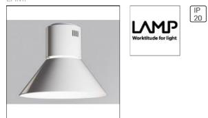
Suspended downlight model STORMBELL 5000 NW FL WH/WH., LAMP brand. Made of shiny white extruded and injected aluminum body with polycarbonate opal ring. Model for COB with neutral white color temperature and control gear included on white decorative rose. Flood aluminum reflector. Insulation class I.
