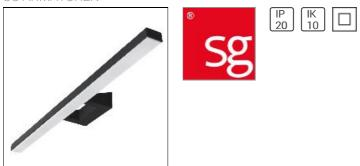
Slim bathroom luminaire for easy mounting over mirror. The luminaire has integrated LED and long life. Light distribution Direct Light technic LED 28W 2700K Ra>90 SDCM 3 L70/B10 >50,000 hrs Control/Dimming Trailing edge dimming Protection Class II IP44/IP20 IK10 Materials and finish Housing: Aluminium Colour: Black (RAL 9004) Optics: UV-stabilized polycarbonate Mounting/Connection Surface, Indoor Screwless terminal block Max. luminaires per circuit breaker: B10: 12, B16: 19, C10: 14, C16: 23
