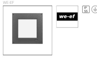
IP55, Class I. IK10. Marine-grade, die-cast aluminium alloy. 5CE superior corrosion protection including PCS hardware. Silicone rubber gasket. Polycarbonate main lens. Two cable entries. Factory installed LED circuit board. Integral EC electronic converter. A pre-installation blockout is available and recommended for mounting in concrete walls.
