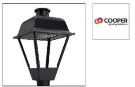
Die-cast aluminum construction; IP66 rated; 3G vibration rated, Up to 141 lumens per watt, Lumen range: 2,000 - 11,000; 9 lumen packages, 120-277V 50/60Hz, 347V 60Hz or 480V 60Hz operation, Greater than 98% lumen maintenance after 60,000 hours at 40°C, Self-aligning poletop fitter for 3" O.D. pole tops or vertical tenons
