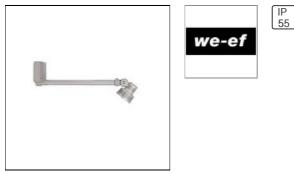
IP55. Marine-grade die-cast aluminium alloy except outreach arm which is extruded. 5CE superior corrosion protection including PCS hardware. Silicone rubber gaskets. Safety glass lens. Anodised aluminium reflector. Two cable entries. Knuckle permits 350° horizontal and 90° vertical aiming of optics.
