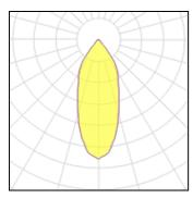
Lamp flux 753 lm Total flux 548 lm Luminous efficacy 126 lm/W Total power 6 W CCT 2700 K CRI 90 1 x LED Nominal lamp power 6 W LOR 73% 753 lm Total flux 548 lm Lamp flux 6 W Luminous efficacy 126 lm/W Total power CCT 2700 K CRI 90 1 x LED LOR Nominal lamp power 6 W 73% Lamp flux 753 lm Total flux 548 lm Luminous efficacy 6 W 126 lm/W Total power CCT 2700 K CRI 90
