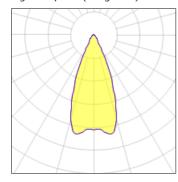
Lamp type LED CCT 3000 K Nominal lamp power 31 W CRI 90 Total flux LOR 100% 2400 lm Luminous efficacy 77 lm/W Total power 31 W
