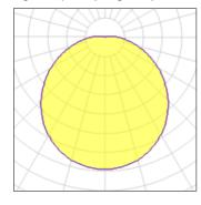
Lamp type Nominal lamp power Total flux Luminous efficacy LED 24 W 2200 lm 92 lm/W CCT
