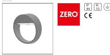
Finish: Painted die-casted aluminum, anthracite grey (RAL 7016) or silvergrey. Prismatic diffuser. LED info: Luminaire Luminous Flux 210LM. Effect 5W CCT 3000K. SDCM 3. CRI >80 Installation: On wall. Connection: Terminal block 5x4mm2. Design: Holscher Design 2016.
