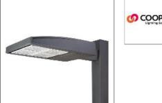
Choice of 16 high-efficiency, patented AccuLED Optics™, Lumen packages range from 4,200 - 80,800 (34W - 640W), Available in 2200K, 2700K, 3000K, 3500K, 4000K, 5000K or 5700K CCT, -40°C to 40°C operating range, optional 50°C high ambient, 120-277V 50/60Hz, 347V 60Hz or 480V 60Hz operation, IP66 rated housing and light square, 3G vibration rated, Pole, mast-arm or wall-mounted configurations, Fiveyear warranty
