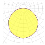
LED Lamp type Nominal lamp power 12 W Total flux 4825 lm Luminous efficacy
