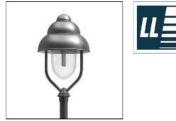
For medium and high light requirements, mounting height 3.80 m. - Impact-resistant clear polycarbonate attachment, UV-stabilized, -Aluminium luminaire body, inside finished in white paint, outside painted in colour - Aluminium unit carrier, painted white - Adapter jack connection -Available in any RAL or DB colour without surcharge - Scope of supply includes fork bracket,post dia. 76 mm (for 3,80 m mounting height) and ornamental ring, painted
