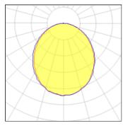
CCT 4032 K Lamp type LED Nominal lamp power 38.16 W CRI 80 100% Total flux 4512 lm LOR Luminous efficacy 118 lm/W Total power 38.16 W
