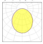
Lamp type LED CCT 4032 K Nominal lamp power 38.16 W CRI 80 Total flux 4512 lm LOR 100% Luminous efficacy 118 lm/W Total power 38.16 W
