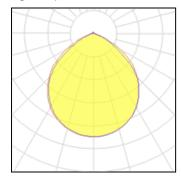
1 x LED Nominal lamp power 25 W Lamp flux 2500 lm Luminous efficacy 100 lm/W 6000 K CCT CRI
