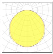
CCT 4000 K Lamp type LED Nominal lamp power 25 W CRI 80 100% Total flux 1950 lm LOR Luminous efficacy 78 lm/W Total power 25 W
