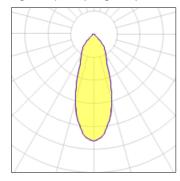
Lamp type LED CCT 3000 K Nominal lamp power 7.5 W CRI 80 Total flux LOR 100% 540 lm Luminous efficacy 72 lm/W Total power 7.5 W
