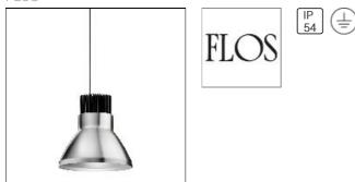
Suspended ceiling-mounted luminaire with LED light source (4 metres maximum distance to ceiling). Power supply source integrated into luminaire housing. Reflector not included; supplied separately.
