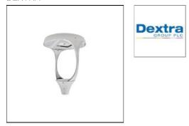
Opus 360 - IP65 Column top mounted open area luminaire, matt grey weather resistant paint finish. Diecast aluminium housing, 50-60mm spigot. Options: BL - Black Body C73 - CRI 70 3000K OPU36 60MM ADAPTOR - Opus360 60-76mm Spigot
