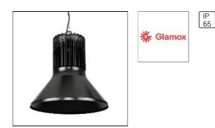
Light source: LED Lumen out: 9669 CRI: 80 Colour temperature: 4000 Total effect: 81 Lumen per watt: 119 Optic: WB Driver: HF/DALI IP class: 65
