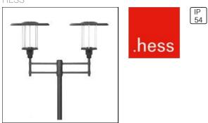
Round luminaire canopy made of aluminium, plain coloured. Support elements made of stainless steel. Cylindrical luminaire enclosure made of PMMA. Round luminaire body made of aluminium. 10.35701.2V001 PARALLEL ROHRE Bracket MADRID 600/600-2 double Made of galvanised steel Overhanging 450 mm on each side Spigot pole ø 76,1 mm Colour: DB 703 or all RAL- (classic- single shades), Hess-DB and Hess-Glimmer-colours. RAL pearl-mica-metallic-shades on request.
