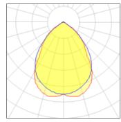
Lamp typeLEDCCTNominal lamp power21 WCRITotal flux2300 lmLORLuminous efficacy110 lm/WTotal power
