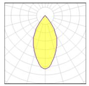
Lamp type Nominal lamp power Total flux Luminous efficacy LED 27 W 2275 lm 84 lm/W CCT CRI LOR Total power 3100 K
