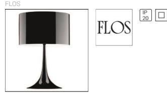
Table/desk fixture providing diffused lighting. Spun metal frame and diffuser, die-cast aluminum diffuser support arms and lamp-holder support, painted for white, balck and brown versions, or polished and transparent painted for aluminum version. White, injection-molded polycarbonate diffuser supports. Sandblasted pressed glass upper diffuser screen. ON/OFF switch and 0-100% dimmer fitted on the bipolar power cord, length 1700 mm. Net weight 4,3 kg.
