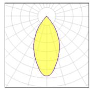
Lamp type Nominal lamp power Total flux Luminous efficacy LED 27 W 2400 lm 89 lm/W CCT CRI LOR Total power 3100 K
