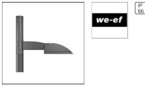
IP66, Class I. Marine-grade die-cast aluminium alloy. 5CE superior corrosion protection including PCS hardware. Silicone CCG® Controlled Compression Gasket. Safety glass lens. Control gear on hinged and 'no tool' removable gear tray. Anodised aluminium reflector, for beam efficiency and glare control. Recommended mounting height 2,5-10,0 m, depending on lamp type selected.
