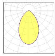
Lamp type LED CCT 3000 K Nominal lamp power 3.2 W CRI 90 Total flux LOR 100% 298 lm Luminous efficacy 93 lm/W Total power 3.2 W
