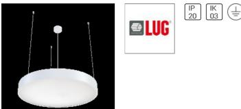
Decorative pendant luminaie for LED light sources. Mounting: suspended, on wire suspension (included) Body: formed aluminum profile, plastic, steel sheet Power supply efficiency: >90% Power: 220-240V 50/60Hz Includes light source: yes Lifetime (L80B10): 100 000 h Operating temperature range: 0°C ... +35°C Warranty: 5 years Application: offices, conference rooms, reception desks, shopping centers, car showrooms, boutiques
