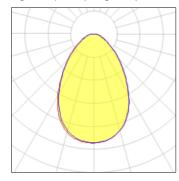
Lamp type LED CCT 3000 K Nominal lamp power 12.5 W CRI 80 Total flux LOR 100% 1220 lm Luminous efficacy 98 lm/W Total power 12.5 W
