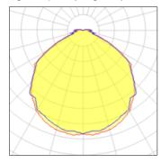
LED CCT 3000 K Lamp type Nominal lamp power 2 W CRI 80 Total flux LOR 100% 186 lm Luminous efficacy 93 lm/W Total power 2 W
