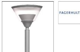
Installation Luminaire for assembly on a post, with post top Ø 60 mm or Ø 76 mm. Connection Supplied with 5 m cable 2x1.5 mm<sup>2</sup>. Design Body of cast aluminium and stainless steel details. Shade of UV-stabilised, clear polycarbonate. Re-lamping from the top. Driver in the luminaire and fuse insert integrated in the post. Louvre Acrylic louvre. Reflector Reflector of anodised aluminium. Standard colour Anthracite
