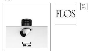
Led recessed luminaire for indoor application. Self extinguishing ceramic or engineering plastic lamp holders, with single-pole, transparent electric wires with double Teflon insulation. Aluminum body, placed above the lamp holder, black thermoplastic and 4 mm tempered glass screen-support ring. Die-cast aluminum alloy body, cover and adjustable lamp support, powder-coated white, grey or black. 220-240V, 50-60Hz power supply included.
