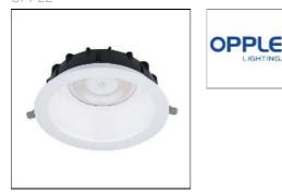
Housing: AL; Mounting ring: white Installation: Recessed mounted; Dimensions: 58\*Φ165mm; Ceiling cutouts: φ140-150mm Power:11W; Efficacy : 109Lm/w Colour temperature: 4000K; Colour rendering: RA80 Total luminous flux of luminaire: 1200Lm Beam angle: 70°; Glare control: UGR22 Service life: 60,000h at 70% luminous flux Degree of protection: IP20, IP44 for exposed part; Class of protection II; Mains voltage: 220-240V/50-60Hz; Remark : also can offer DALI control and Bluetooth
