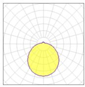
CCT 3000 K Lamp type LED Nominal lamp power 35 W CRI 80 LOR 100% Total flux 3500 lm 100 lm/W Luminous efficacy ULOR 12% Total power 35 W
