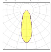
Lamp type LED CCT 3000 K Nominal lamp power 7.5 W CRI 80 Total flux LOR 100% 470 lm Luminous efficacy 63 lm/W Total power 7.5 W
