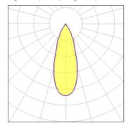
LED CCT 3000 K Lamp type Nominal lamp power 26 W CRI 79 Total flux LOR 100% 1365 lm Luminous efficacy 52 lm/W Total power 26 W
