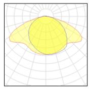
1 x Metal halide lampNominal lamp power7Lamp flux7200Luminous efficacy63 lnCCT300CRI200
