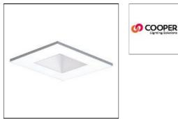
Die cast trim ring with metal baffle, Mounting methods include friction clips, 15° tilt, 36° orientation in housing, Trim ring finishes in a wide variety of colors, Baffle available in a various kinds of finishes, Showerlight trims with wet location listing
