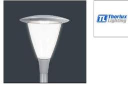
Stylish IP66 rated pole top amenity luminaire with aluminium cast body and spigot adaptor. UV stabilised polycarbonate cover rated IP66 and IK10. Integral high quality LED driver. Applications: car parks, amenity areas and hospital estates.
