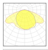
1 x High pressure sodium vapour lampNominal lamp power70 WLamp flux5600 lmLuminous efficacy52 lm/WCCT2000 KCRI25
