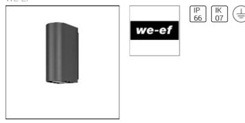
IP66, Class I. IK07. Marine-grade, die-cast aluminium alloy. 5CE superior corrosion protection including PCS hardware. Silicone rubber gasket. Safety glass lens. Two cable entries. Integral EC electronic converter. CAD-optimised optics for superior illumination and glare control. OLC® One LED Concept. Factory installed LED circuit board. 1-10V or DALI interface on request.
