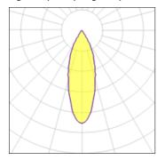
Lamp type Nominal lamp power Total flux Luminous efficacy LED 21 W 1850 lm 88 lm/W CCT
