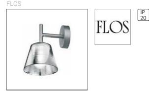
Wall sconce providing diffused lighting.Injection-molded polycarbonate external diffuser completely finished with high-vacuum aluminization process.Gray painted die-cast aluminum diffuser and lamp support. Gray painted, injection-molded polycarbonate wall fitting and rose. Net weight 0,5 kg
