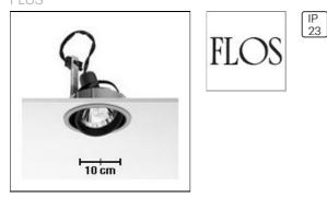
Luminaire for halogen and high-pressure discharge lamps. Injection-moulded aluminium reflector body with powder-coated finish. Lamp support with die-cast aluminium, black powder-coated heat dissipating element. Thermoplastic recessed ring and screening ring, die-cast aluminium, black powder-coated anti-glare ring. 4 mm. tempered glass cover. Stainless steel fixing brackets.
