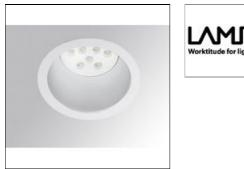
Round recessed DOMO 220 G2 2000 NW downlight, LAMP brand. With external ring in white lacquered die-cast aluminium. Model for MID-POWER LED, neutral white colour temperature and control gear included. Reflector designed by the optical concept named REDIL (Direct Emission LED Reflector), which consists of a two-phase reflection. Insulation class II.
