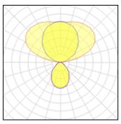
Lamp typeLEDNominal lamp power68 WTotal flux9400 lmLuminous efficacy138 lm/W
