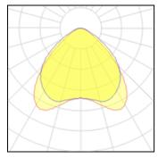
CCT 4000 K Lamp type I FD Nominal lamp power 165 W CRI 80 Total flux 25484 lm LOR 100% Luminous efficacy 154 lm/W Total power 165 W
