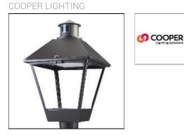
Aluminum housing, top, and base, Greater than 98% life at 60,000 hours (40°C) (LED), Up to 140 lumens per watt, Lumen packages ranging from 2,000 – 11,000 lumens, Self-aligning pole-top fitter fits 2-3/8" and 3" O.D. tenons, Optional NEMA photocontrol receptacle, Five-year warranty (LED)
