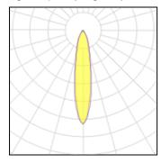
LED CCT 4000 K Lamp type Nominal lamp power 14.6 W CRI 90 Total flux 1330 lm LOR 100% Luminous efficacy 91 lm/W Total power 14.6 W
