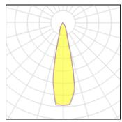
1 x LED Nominal lamp power 52 W LOR 71% Lamp flux 8980 lm Total flux 6371 lm Luminous efficacy 173 lm/W Total power 56 W CCT 4000 K CRI 80
